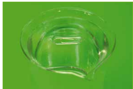
Surface tension of water (cohesion)
