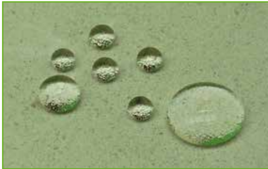
Hydrophobing : Making the building material water repellent
