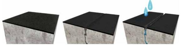
1. Elastic but not crack bridging: The waterproofing layer does not withstand the permanent water pressure.
