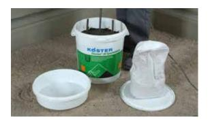
The KÖSTER Deuxan<sup>®</sup> 2C bucket has an insert which contains a bag with the powder component. The powder component is slowly mixed into the bitumen component using a slow rotating stirring device. Mixing time is 3 minutes.
