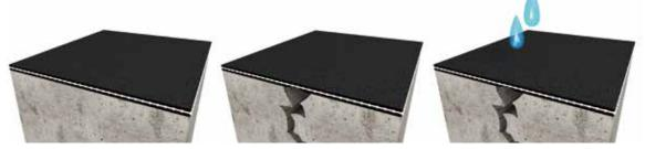
3. Crack bridging due to an embedded mesh. The mesh separates the top waterproofing layer from the crack and helps significantly to withstand permanent water pressure.
