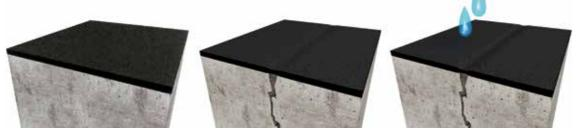
2. Crack bridging waterproofing: In this case due to elasticity and layer thickness. The waterproofing layer withstands permanent water pressure.
