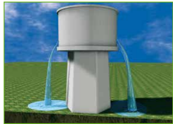
Filled water tanks cannot be accessed from the inside to apply a waterproofing layer. For an uninterrupted usage, waterproofing from the outside (negative side) is necessary.
